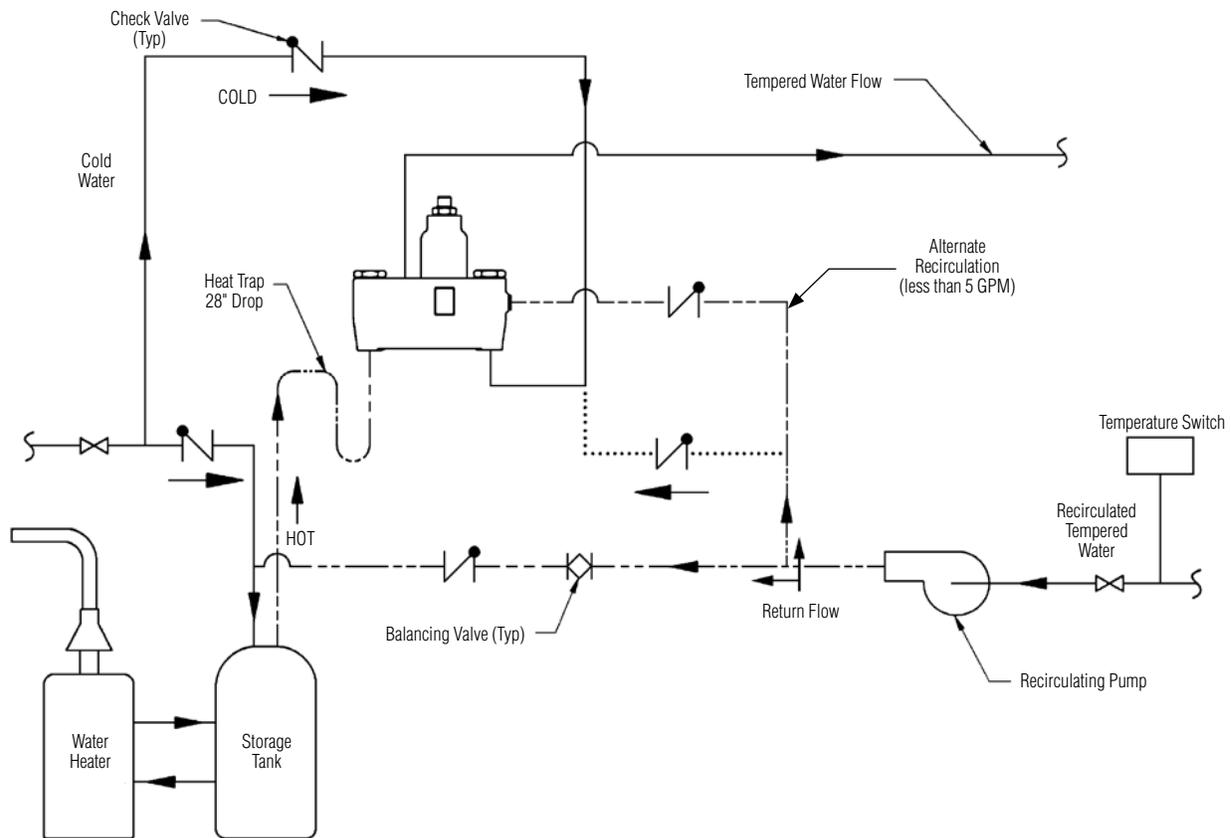
1. Turn off the recirculating pump and turn on the water supply at emergency fixture (a water flow rate of 10-15 GPM is required).
